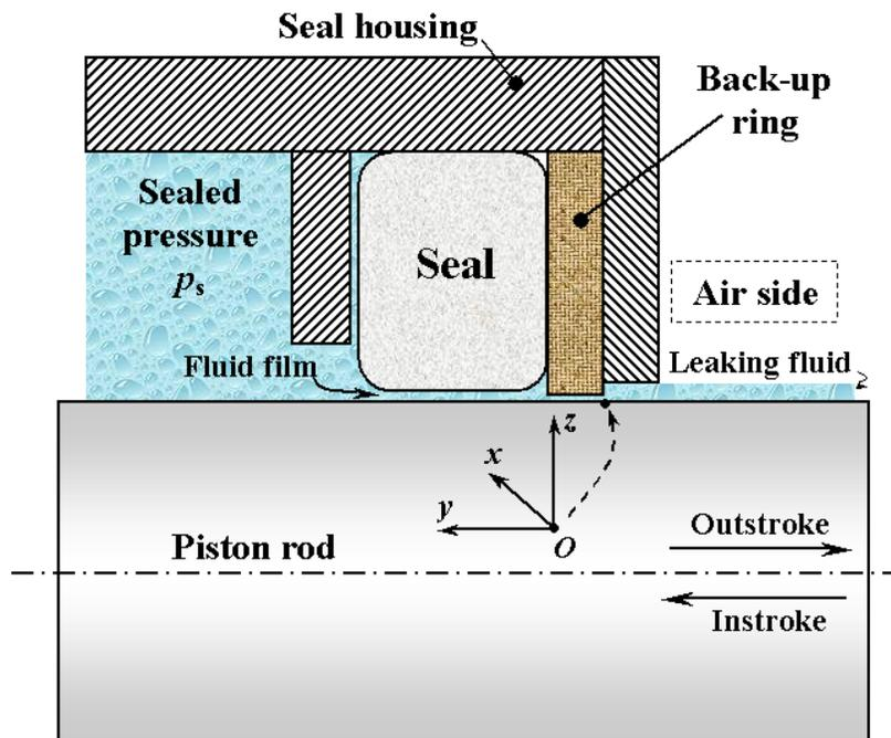
Figure 13. Schematic of rectangular elastomeric seal with back-up ring in a linear hydraulic actuator (only the upper half of the seal, ring and housing shown)
