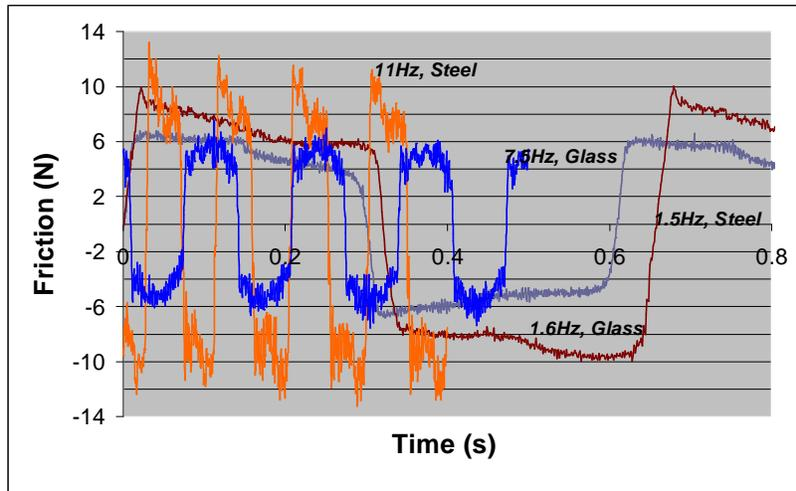
Figure 8. Friction measurements at various reciprocating frequencies and glass-plate roughness from the rig pictured in Fig. 7 (from [36, 91])
