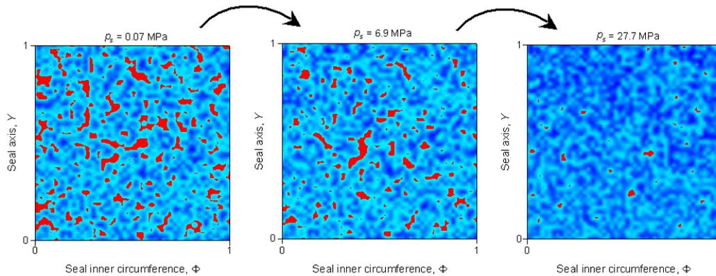
Figure 14. Film contour maps from the rough contact simulation of rod seal on piston rod. Lighter shaded areas indicate thinner film and red are areas of solid contact. Notice the partial film collapse at low sealed pressure  $p_s$  (left image)
