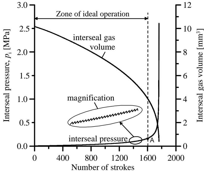
Figure 18. Variation of interseal pressure and gas volume with the number of strokes in a tandem seal arrangement of identical, rectangular, rounded elastomeric seals [40]
