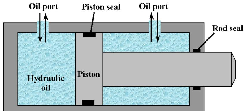
Figure 1. Typical hydraulic seals in a linear hydraulic actuator
