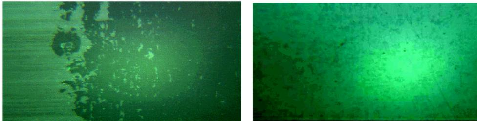
(a) Dry conditions (O-ring, 1 mm cross section). (b) Wet conditions (dark spots represent contact).
