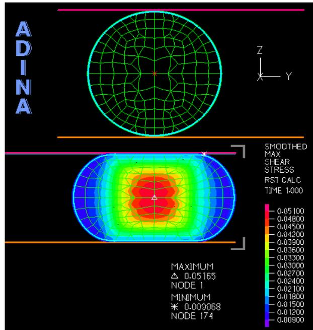
Figure 12. FEA example of a rubber O-ring pressed between two rigid, frictionless plates; original and deformed mesh shown with maximum shear stress distribution
