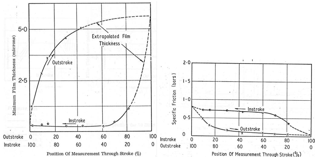
Figure 6. Variation of minimum film thickness and frictional force through the stroke of a reciprocating rectangular rubber seal (from Field and Nau [15])
