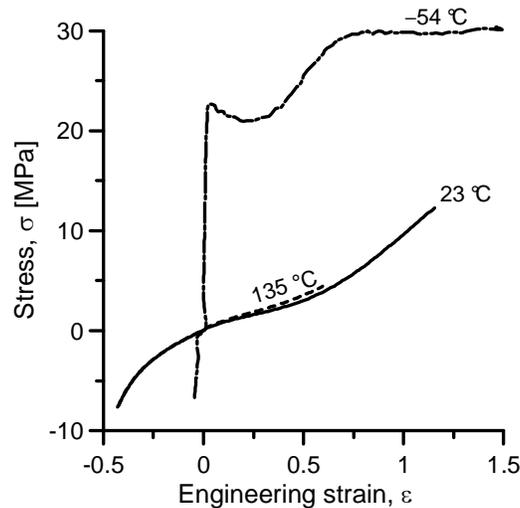
Figure 3. Stress-strain curves of typical elastomer for hydraulic seals [3, 5, 6] (results obtained from Trelleborg Sealing Solutions in England). The glass transition temperature of this elastomer is  $-47\text{ }^{\circ}\text{C}$
