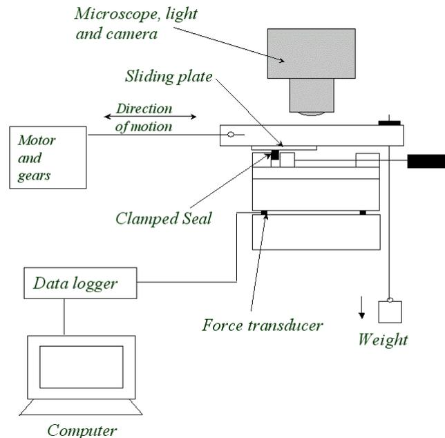
Figure 7. Reciprocating rig for monitoring the sealing interface and performance testing [36, 91]
