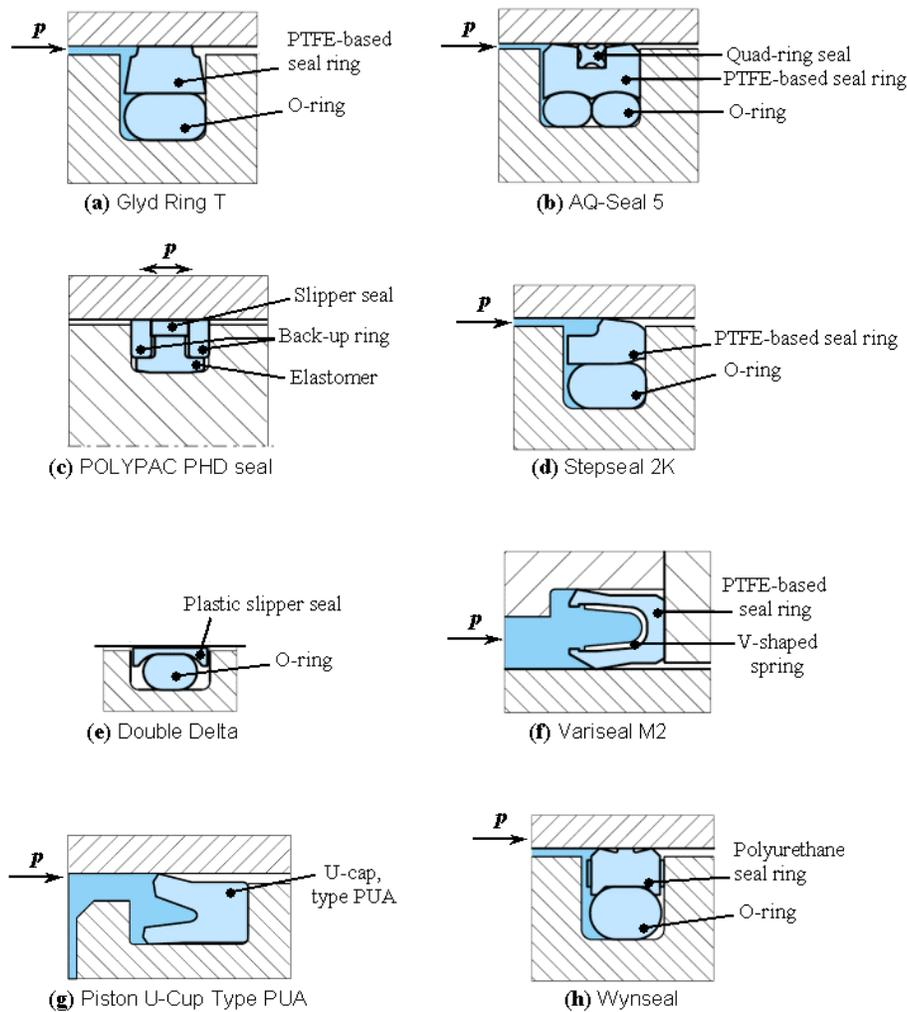
Figure 5. Examples of piston seals (compiled from catalogue [56])
