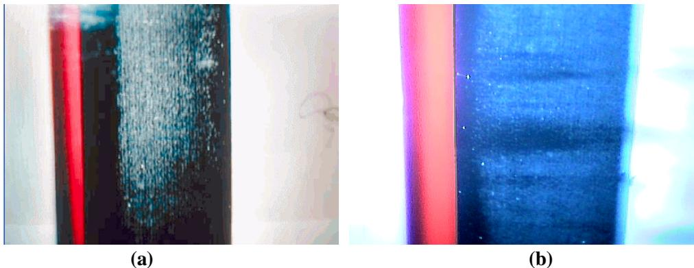
Figure 11. Sealing contact (sealed fluid on the left side of each image) from the rig in Fig. 10 [91]. (a) Nearly zero sealed pressure (thin film); (b) 0.7 MPa sealed pressure (thick, non-uniform film).
