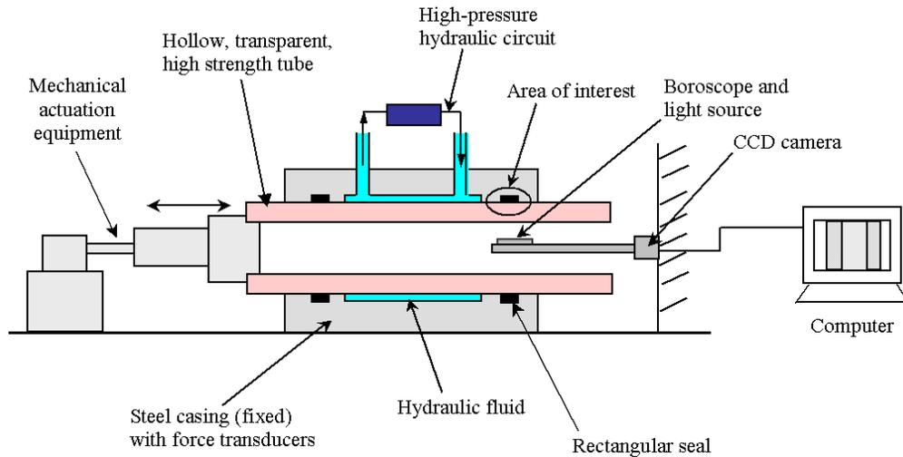
Figure 10. A seal specific rig with glass tube arrangement and boroscope [91, 92]
