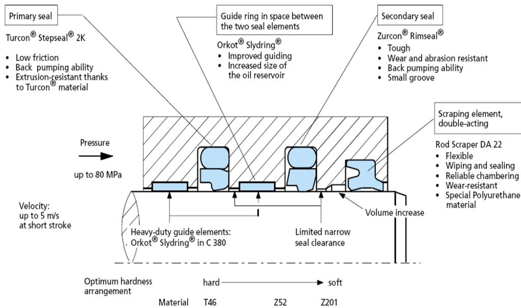
Figure 17. Tandem seal arrangement (courtesy of Trelleborg Sealing Solutions [55])
