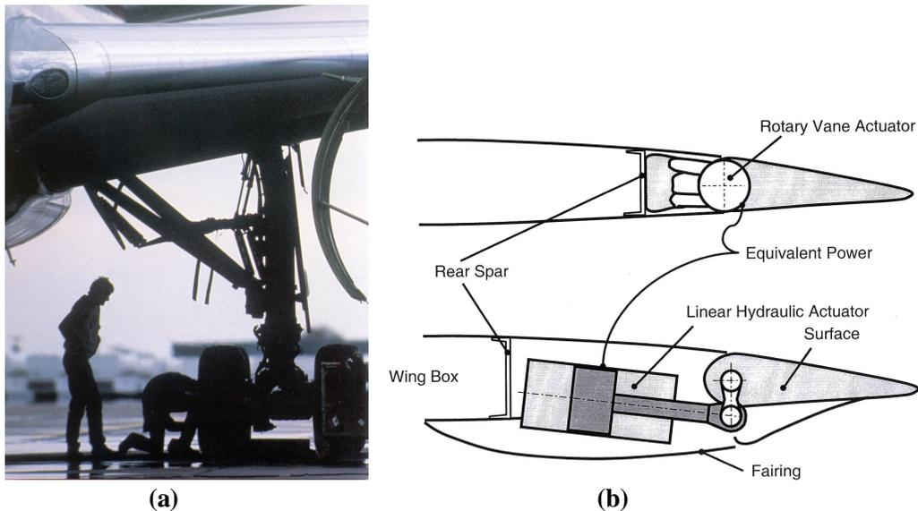
Figure 2. (a) Aircraft landing gear controlled by linear hydraulic actuator; (b) Aircraft wing control surfaces operated via classic linear hydraulic actuator and new rotary vane actuator (drawing courtesy of Smiths Aerospace, UK)
