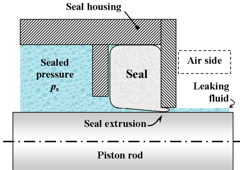
Figure 15. Extrusion of a rectangular, rounded, elastomeric, rod seal (only the upper half of the seal and housing shown)
